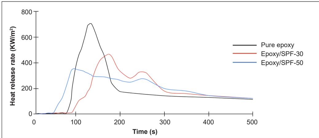
Figure 4. The HRR curves for the samples
