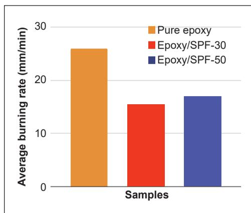
Figure 3. The average rate of burning of composite samples
